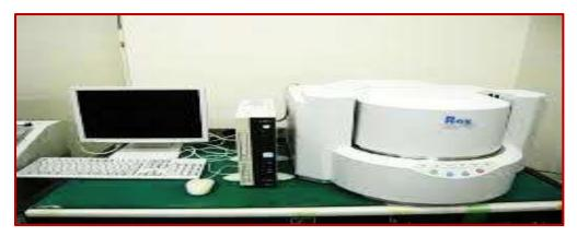
Figure 7: Shinmadzu EDX-720 X-ray spectrometer
